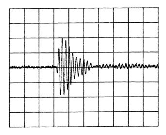
The plot at left shows the time-domain response obtained when one device is driven as a transmitter, and another is used as receiver at a distance of 30 cm. The drive signal comprised a single cycle at 400 V pk-pk. Receiver gain was +26 dB.
