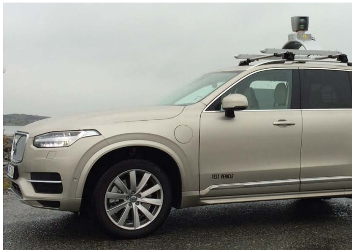
HDL-64E mounted atop Volvo CX-90 self-driving research vehicle. 360° sensor rotates up to 15 Hz. Courtesy www.volvocars.com
