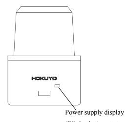
(Blinks during start up and malfunction state)
